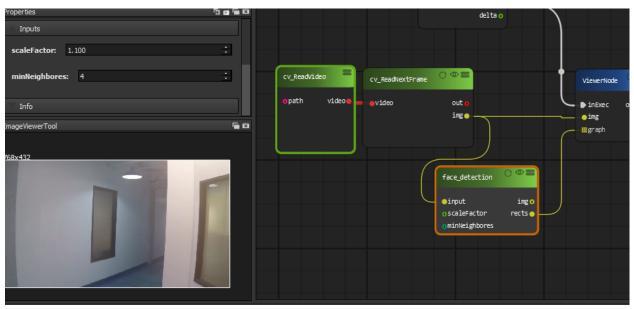
If you want to detect face from the WebCam, just drag a WebCam node to the diagram instead of the ReadVideo node:
