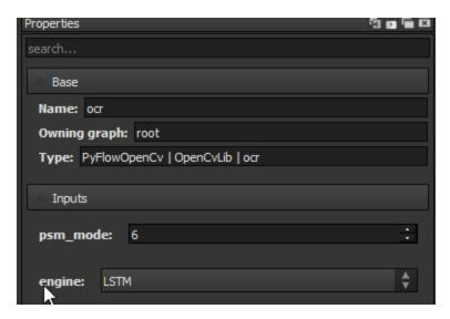
Page Segmentation Mode (-psm). That affects how Tesseract splits image in lines of text and words. Pick the one which works best for you:
